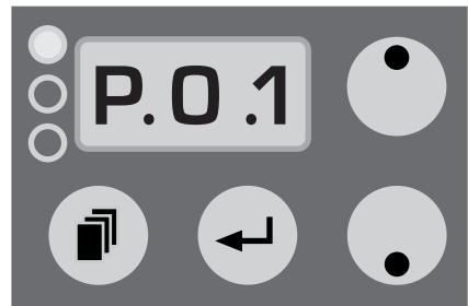
Adjusting of the wait time in minutes (0.1-99)
