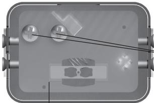
6: Screws for connecting the vaporizer to the connecting pins
