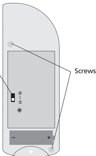
ter that has its internal white switch in position „f2“. See section 4.2 for pairing instructions.
