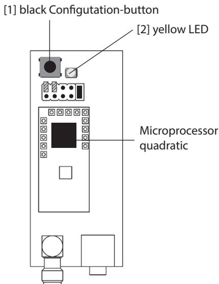
Fig. 6: PCB version 2 - Microprocessor quadratic, fixation all around.
