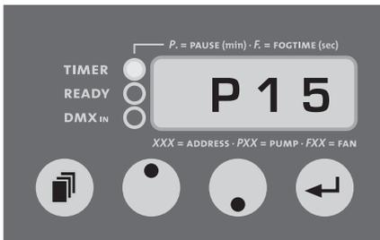
*Adjusting of the output/pump
