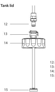
12: Plastic spigot 13: Quick coupling 14: Tank lid 15: Filter
